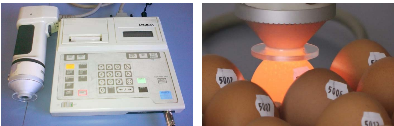
Figure 3: Reflectometer used to measure eggshell color
